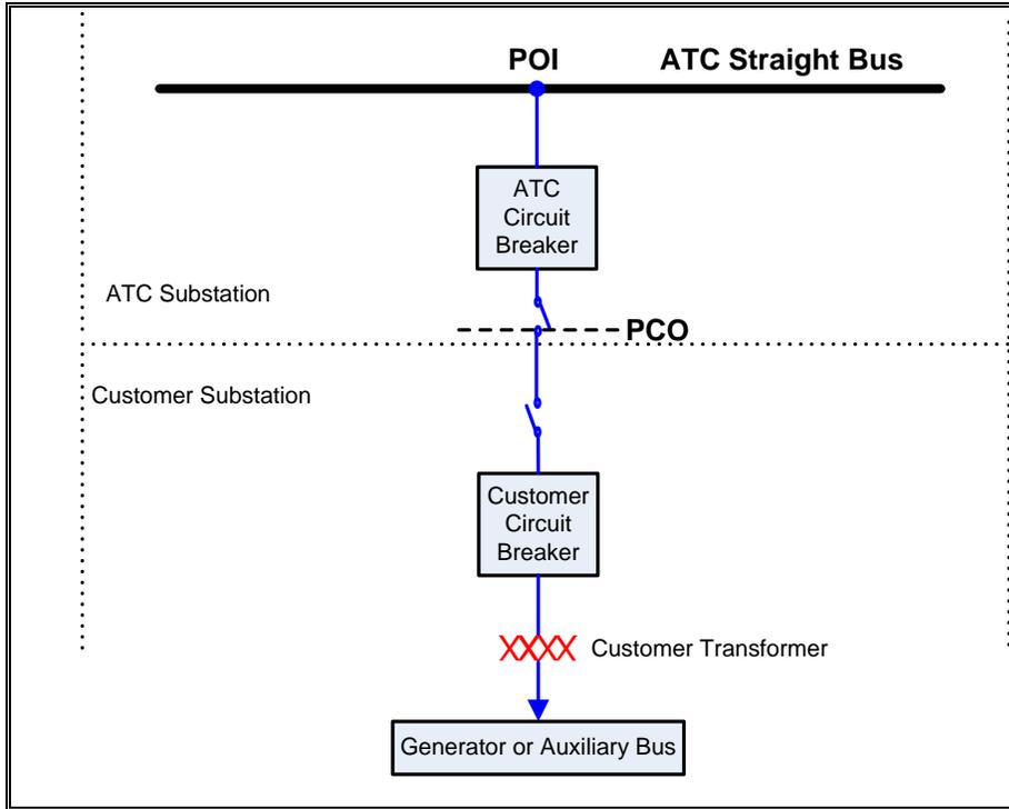
Figure 2 Straight bus configuration
