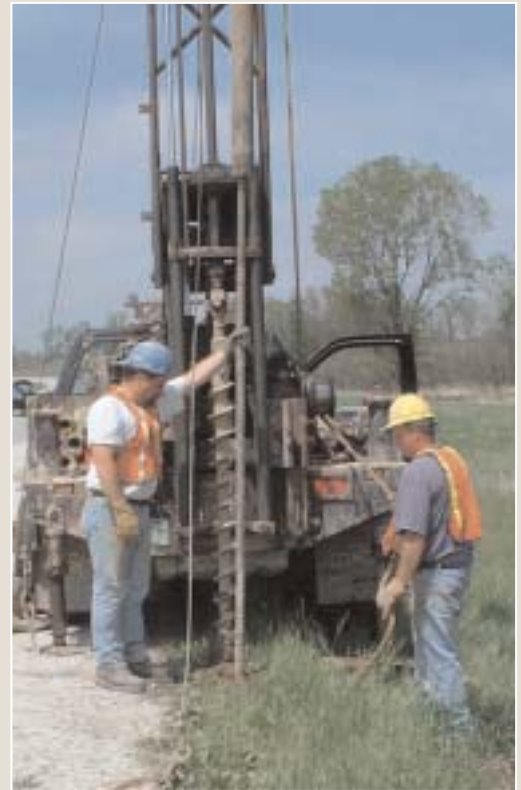
Soiling boring tests being conducted along Hwy. 164 and Hwy. 74 help to determine soil characteristics. The data is used to determine the placement and design of poles that are best suited for the soil conditions.
